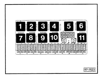
Auxiliary relay carrier, front (under left dash panel)
