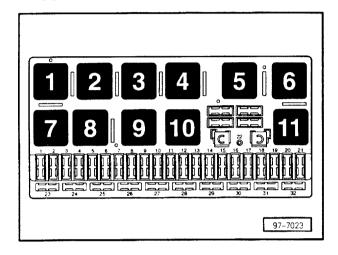
Auxiliary relay carrier, front (under dash panel, left)
